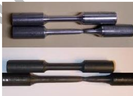
Figure 15: Examples of sample pairs before and after pulling for Al versus Cu test specimens
