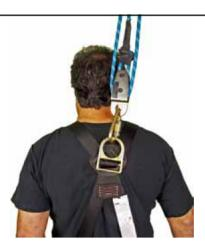
Apply firm tension on the safety rope to maintain a secure hold on the ring. Then pull the rescue rope toward you while holding the telescoping pole in place. This will cause the spring on the SureClip to compress causing the auto locking gate on the carabiner to close.
